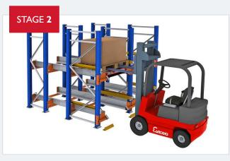
The pallet is then placed at the rail entrance using a forklift truck, supported by the load profiles.
