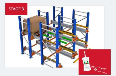
In stage 3, in order for the satellite cart to start loading operations the operator has to give the order via remote control.
