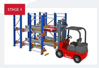
The satellite cart is placed on the lane where you want to operate using a forklift.
