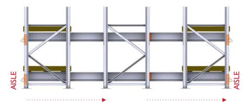
LIFO (Last In, First Out) With this method, the last pallet to enter is the first to leave, so both loading and unloading are done through the same access.
